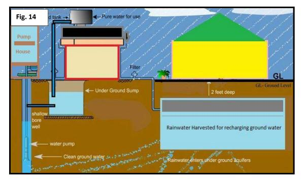
Fig. 14 - Water Circuit Diagram of the Borewell and Rainwater Harvest Utilization in RIE, Bhubaneswar
